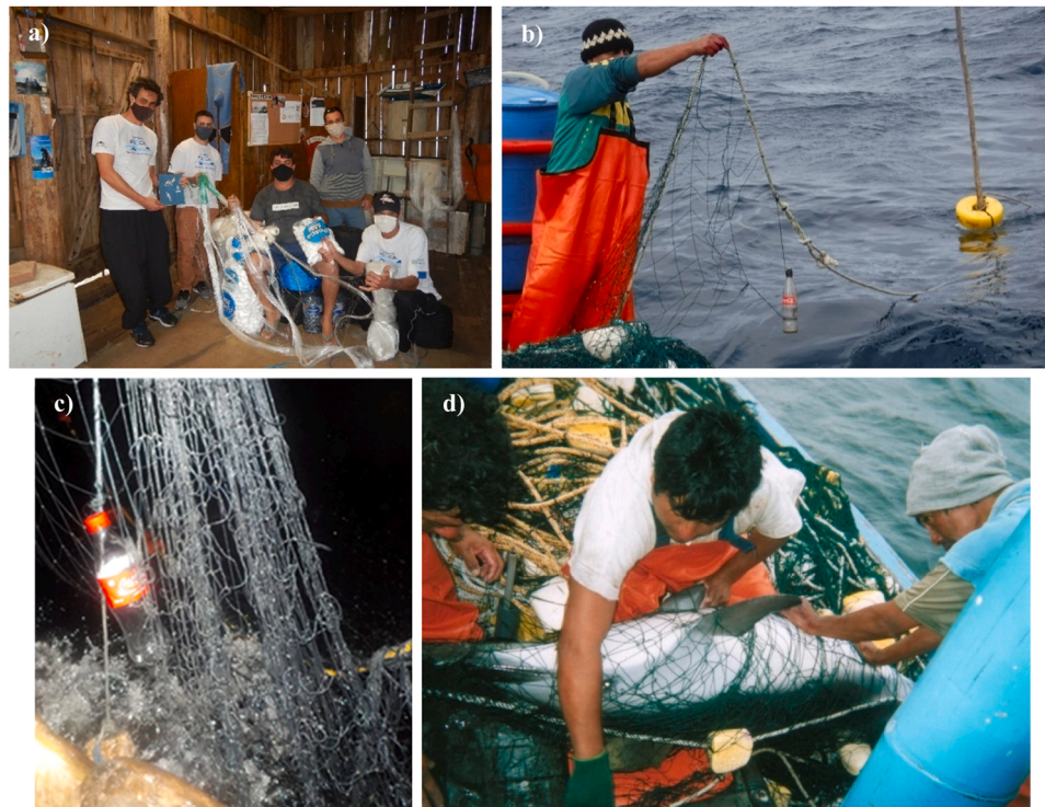
Fig. 3. Up-cycled glass bottle pingers and plastic bottle acoustic reflector trials. a) Workshops were held with fishermen in the targeted fisheries to introduce the project and secure participants. b) glass bottle pinger attached to a surface-set driftnet. c) Plastic bottle acoustic reflector attached to a surface-set driftnet. d) dolphin bycatch in a surface-set driftnet during the trial.
